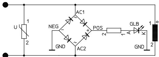
M12x1 – Pin allocation on the valve
