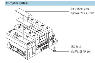
A holder VMPAL-ST-AP-10 (Part No. 561109) with inscription labels (Part No. 18576, IBS-6x10) can be mounted on each sub-base for labelling the valves. Large inscription labels can be attached to the pneumatic interface as an alternative or in addition to the smaller labels.
