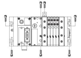
The MPA-L valve terminal is screwed onto the mounting surface using four M4 and two M6 screws or using six M6 screws. The mounting holes are
