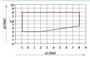
For valves in width 14 mm with code for position function 1-32: NS, KS, HS, DS
