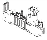
An adjustable pressure regulator can be installed between the sub-base and the valve in order to control the force of the triggered actuator. This pressure regulator maintains an essentially constant output pressure (secondary side) independent of pressure fluctuations (primary side) and air consumption. Standard version:
