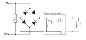
Each solenoid coil is protected with a spark arresting protective circuit as well as against polarity reversal. All valve types are additionally equipped with integrated current reduction. MPA-L valves are supplied with operating voltage in the range 21.6 ...  $26.4 \vee (24 \vee +/-10\%)$ .
