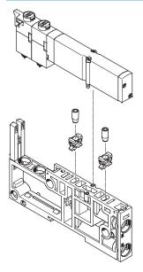
Blanking plate (code L) without valve function, for reserving valve positions on a valve terminal.
