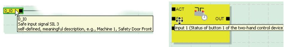
Figure 2-9 Examples of tool tips in the connection editor in offline mode (while editing the safety logic)
