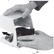
♦ Check that there is no gap of light between the front screen and the housing.
