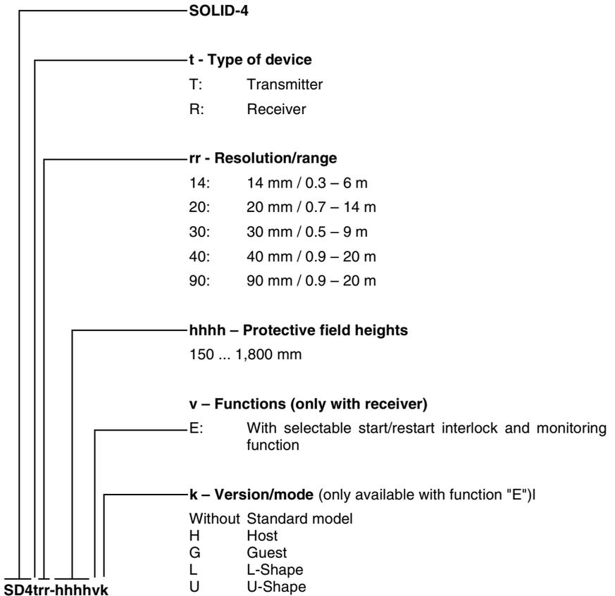
**Fig. 1.3-1:** Selecting a SOLID-4 Safety Light Curtain
