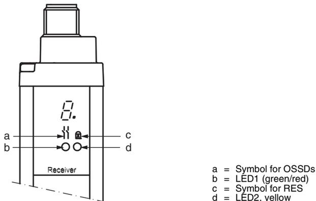
**Fig. 5.2-1:** SD4R-E Receiver status displays
