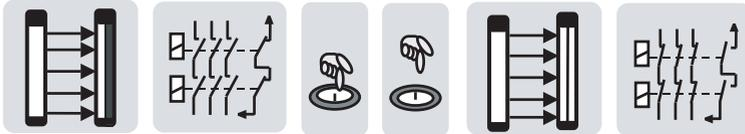
**Fig. 4.2-3:** Contactor monitoring function, combined in this example with RES interlock
