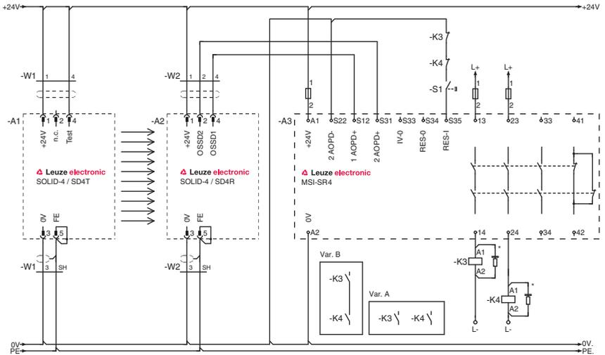
Figure 7.2-4: Receiver SD4R with MSI-SR4
