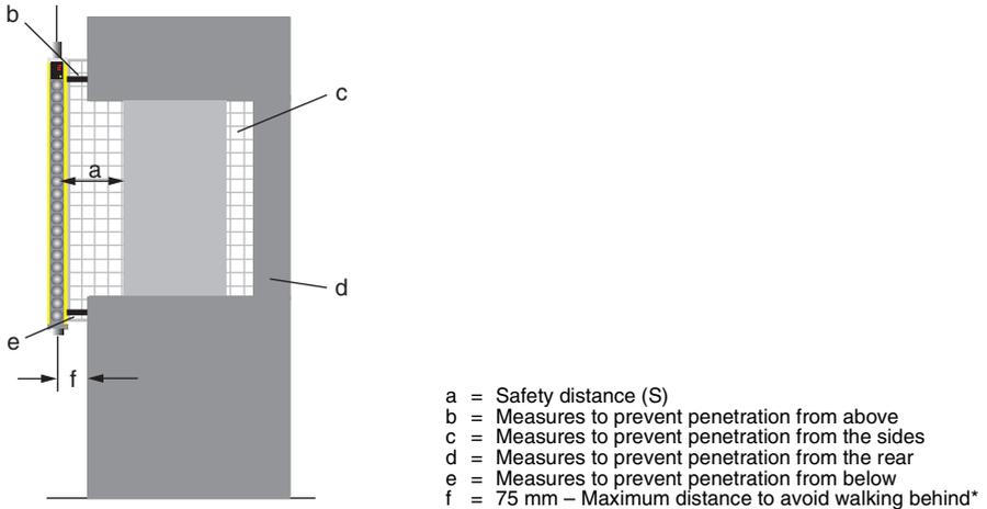
**Fig. 6.1-1:** Safety distance (a) for point of operation guarding
