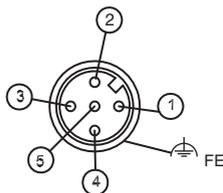
**Fig. 7.1-1:** SD4T 5-pin (view of the pins)
