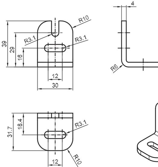
Fig. 11.5-3: Option: L-mounting bracket
