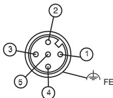
**Fig. 7.1-3:** SD4R 5-pin (view of the pins)
