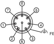
**Fig. 7.1-2:** SD4R-E 8-pin (view of the pins)
