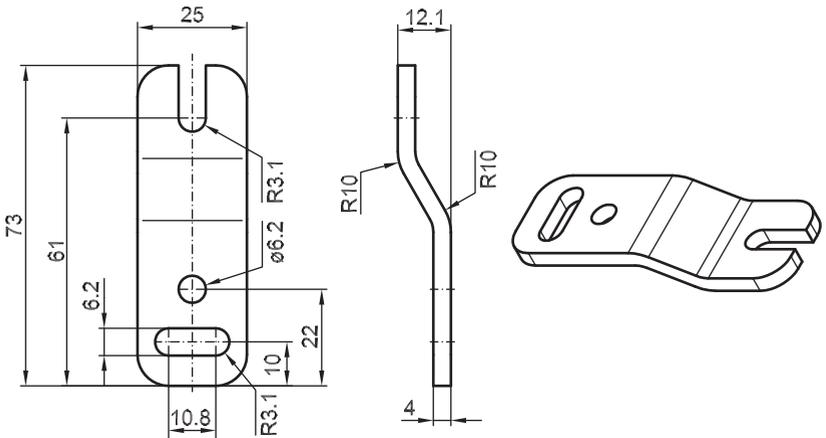
Fig. 11.5-4: Option: Z-mounting bracket
