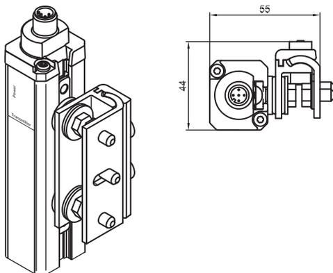
**Fig. 6.4-2:** Swiveling bracket with shock absorber
