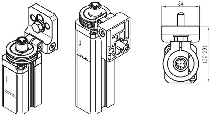
**Fig. 6.4-1:** 360° rotation bracket, mounting examples
