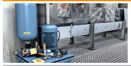
Loose parts become bales of scrap The blank offcuts are compressed into bales of scrap in a high-pressure press.
