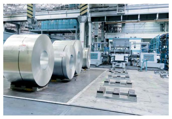
First of all, the blanks are cut from steel coils on a coiling unit. Depending on requirements, these base sheets are edged and may be partially pre-punched.
