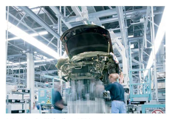
Piece by piece, the complete vehicle is formed from many individual components. Countless bolts fix the assemblies in their places. Clips hold carpets and the interior trim in place. Kilometres of cables and wiring form the vehicle's nervous system.
