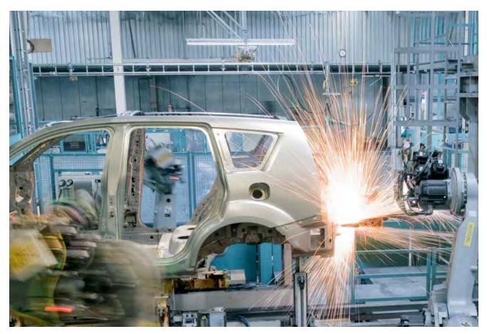
In the body-in-white, up to 200 individual parts and assemblies are put together to form a self-supporting body.
