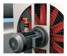
Monitoring of the overall vibration of rotating parts (fans, centrifuges, etc.).
