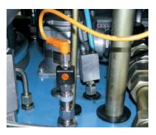
Use of a modular TP transmitter instead of a common head / DIN rail transmitter.
