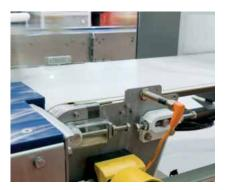
Safe detection of transported parts on a conveyor belt.
