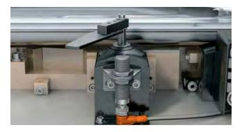
Longer lifetime in welding applications due to anti-adhesive coating.
