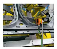
The presence of adhesive pads for noise reduction is checked.
