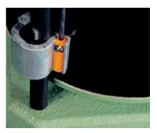
Exact switch point detection on short-stroke cylinders
