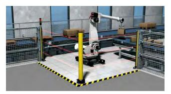
Safety light grids protect the operating area of robots.
