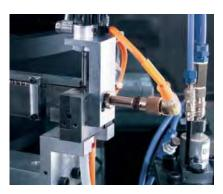
Different metals are safely detected.
