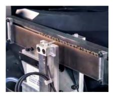
The use of fibre optics allows the detection of objects where space is at a premium.
