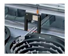
Precise detection of screws in feeder systems.
