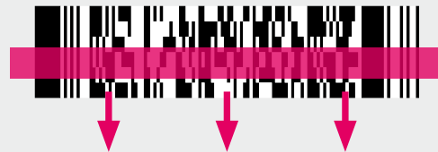
Reading stacked codes with movement of the scanning line over the code.
