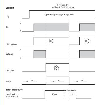
Fault indication is reset when control voltage is switched off, whether the failure is still active or not.
