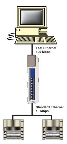
The TSX Quantum Ethernet switch allows operation (with full bandwidth) in both 10 and 100 Mbps speeds, and automatically configures itself to the appropriate speed.
