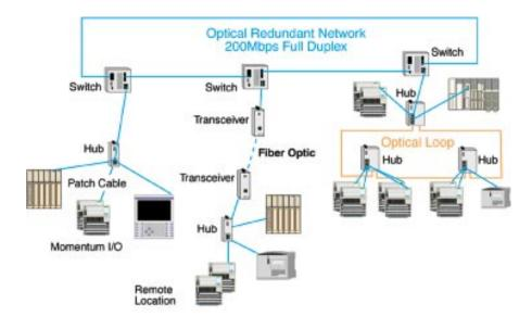
Transparent Factory Ethernet cabling system Hubs
