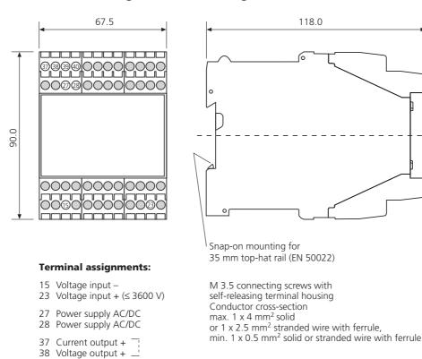
For switchable models and voltage output: Place jumper across terminals 37 and 38
