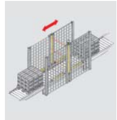
Muting in one/two directions (L-Version and T-Version)
